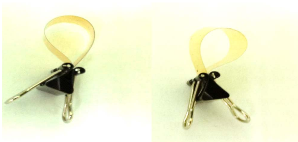
Figure 4. Photographs of (left) P2/DGEBA and (right) P2/CNE. Dimensions of the films: about 6 cm × 0.8 cm × 30 μm. [Color figure can be viewed in the online issue, which is available at wileyonlinelibrary.com .]
